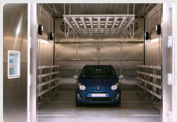
29. Standard Discovery My chamber equipped with sun simulation system. 30. Solar radiation system provided with a special lamp
